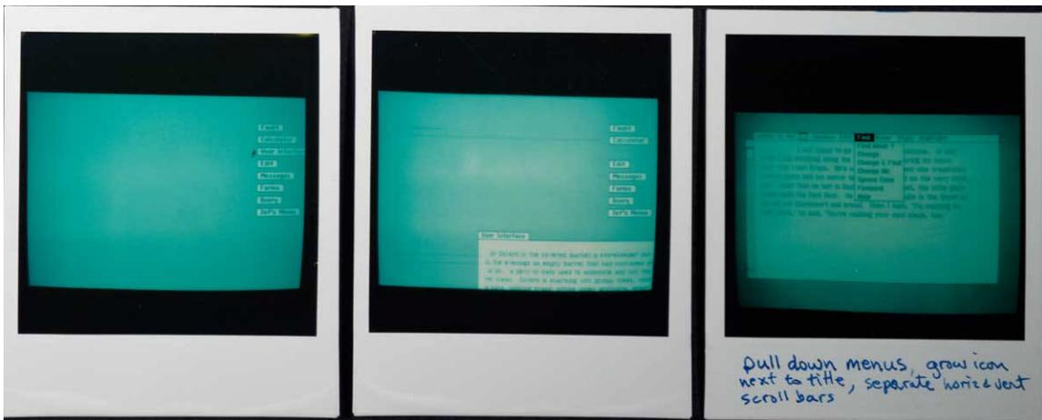
The middle picture shows that windows can be repositioned by dragging a gray outline. We wanted to drag the whole window, like modern user interfaces do today, but the processors weren't fast enough in those days. As far as I know, the NeXTStep was the first system to do it the modern way.
