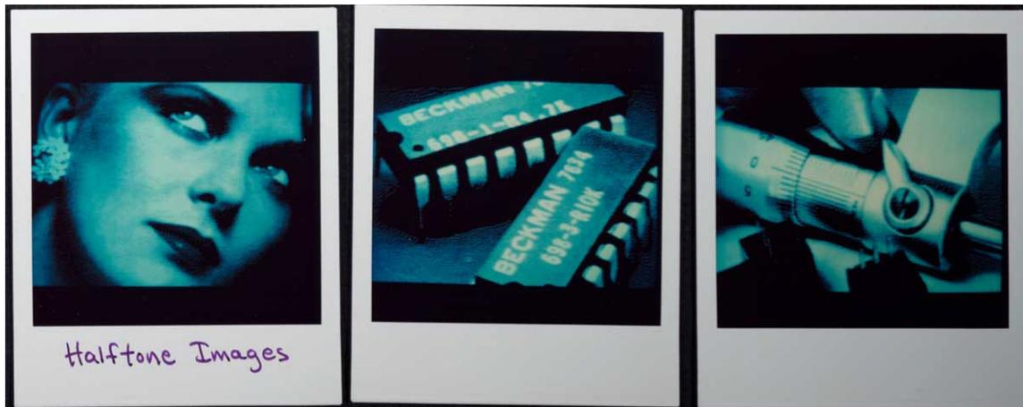
Here are some scanned images, showing off Lisa's impressive resolution for the time, which Bill scanned using a modified fax machine. He was always tweaking the half-toning algorithm, which mapped gray scales into patterns of monochrome dots. Bill had made versions of these for the Apple II that Apple distributed on demo disks, but these higher resolution Lisa versions were much more impressive.
