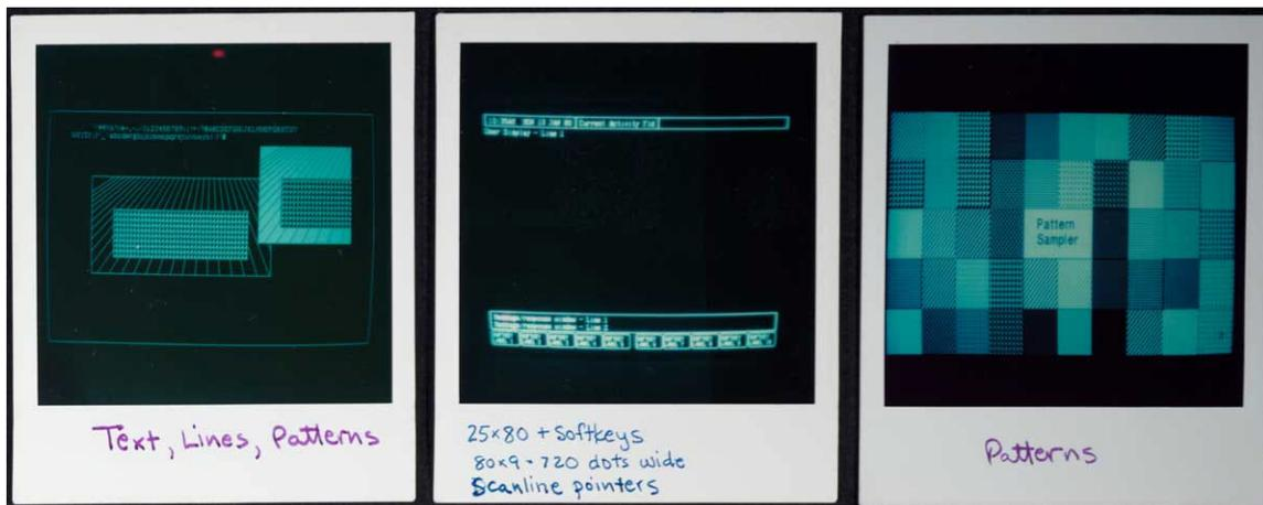
The leftmost picture illustrates the first graphics primitives that Bill wrote for LisaGraf (which was eventually renamed to QuickDraw in 1982) in the spring of 1979, rendering lines and rectangles filled with 8x8 one-bit patterns. The power and flexibility of the patterns are illustrated in the rightmost shot, which were our poor man's substitute for color, which was too expensive (at the required resolution) in the early eighties.
